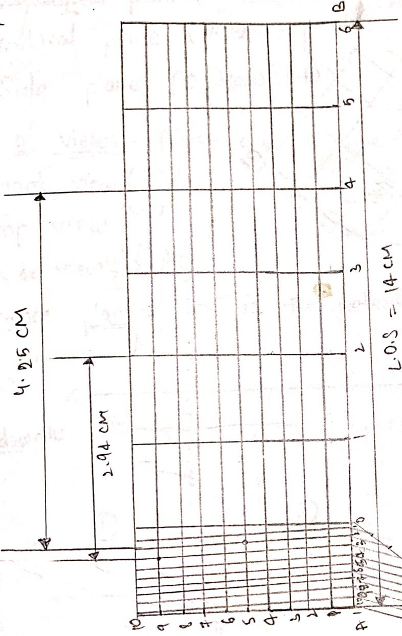
Draw a vernier scale of RF = 4.25 to read centimeters upto 4 meters and on it shows lengths 2.39 m and 0.91 m
