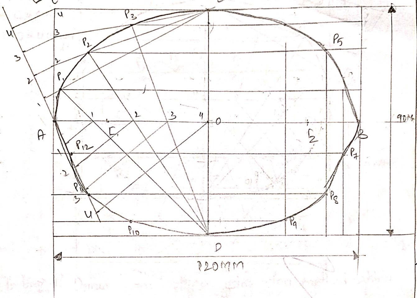
4) Draw an ellipse using oblong method by given minor axis = 80 mm and foci ( $F_1, F_2$ ) = 60 mm
