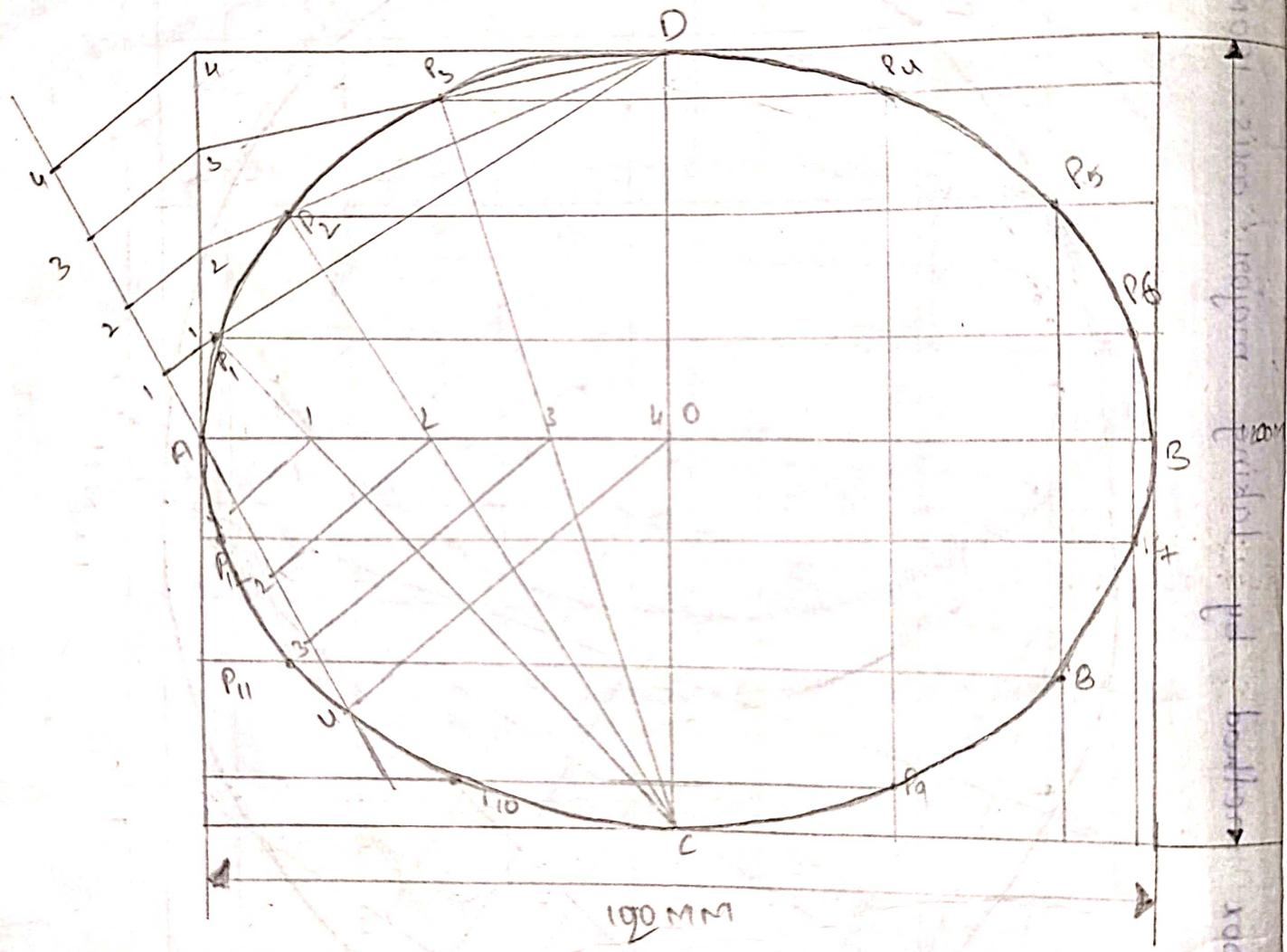
i) Draw an ellipse using oblong method using given major axis = 120 mm, foci = 80 mm.
