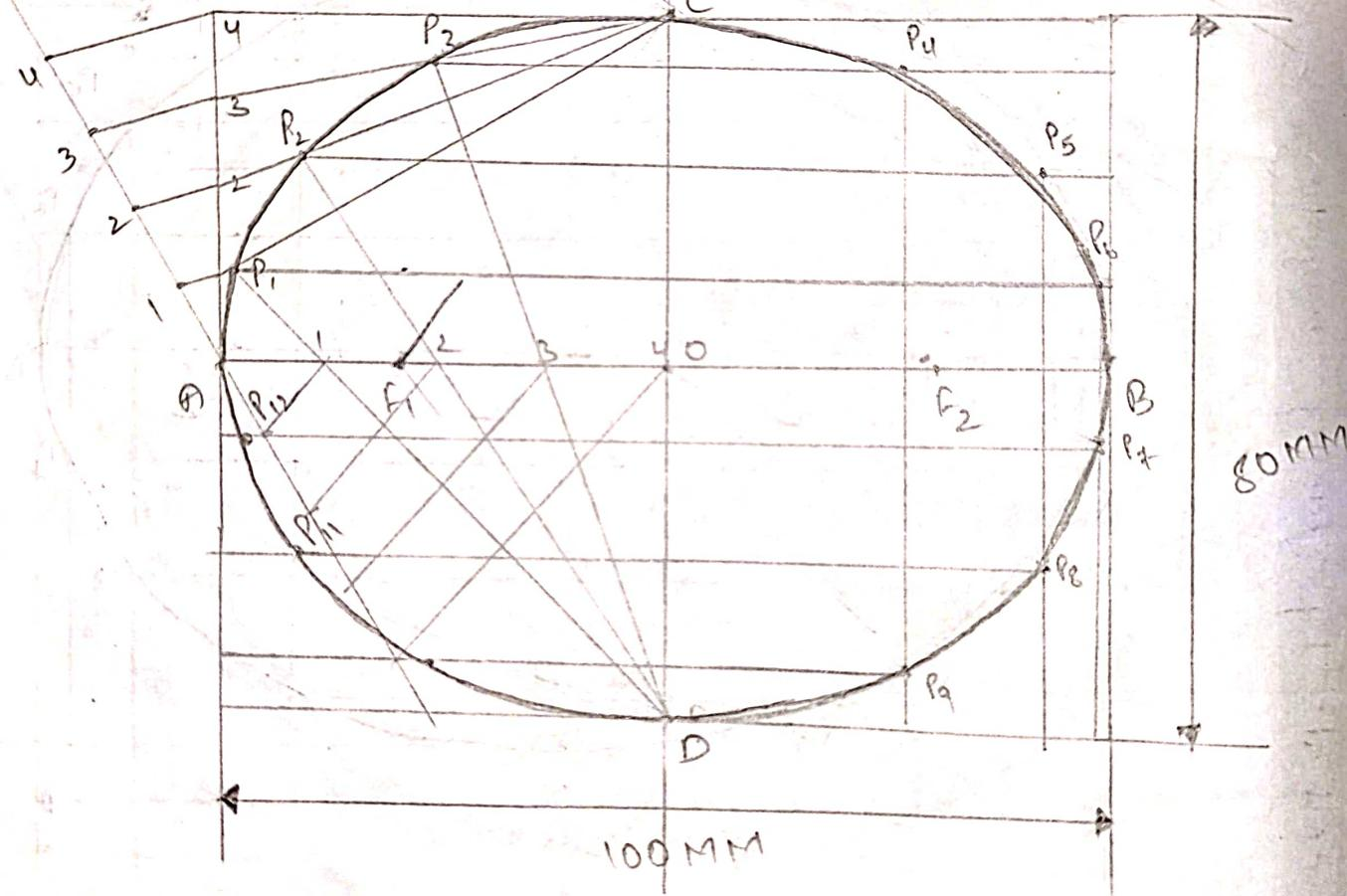
3) Draw an ellipse using box method by given
