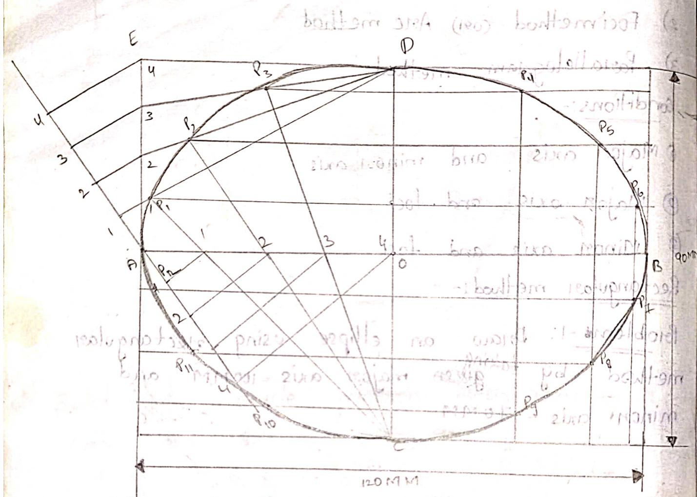
3) Draw an ellipse using box method by taking major axis = 150MM, minor axis = 120MM
