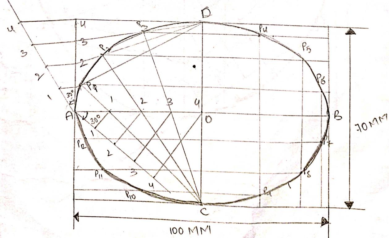
2) Draw an ellipse using oblong method by taking major axis = 120 MM, minor axis = 90 MM
