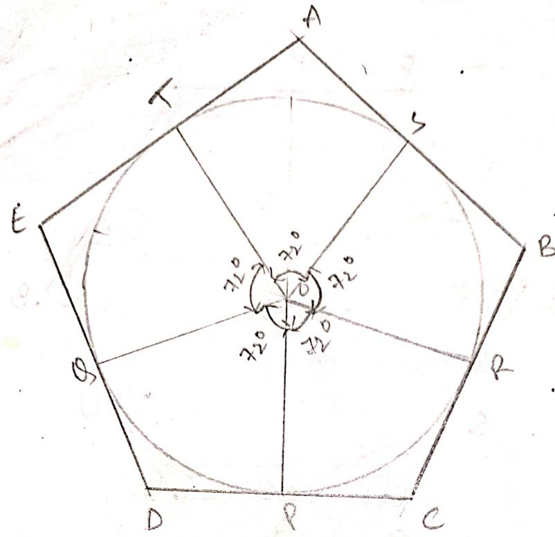
4) Superimpose a circle on a pentagon taking diameter = 70 mm with one side is vertical.
